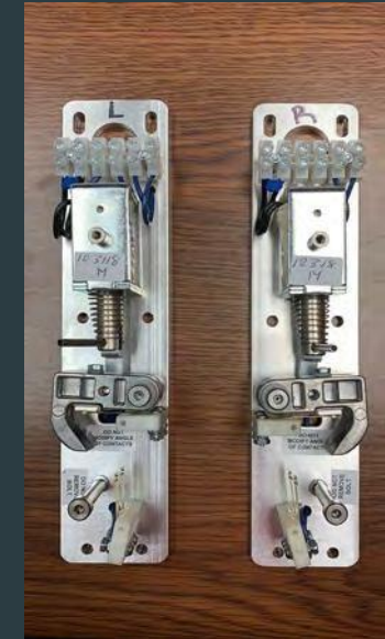
Extrusion, casting, machining, and assembly 6061-T6, A380, Electronics Locking Mechanism
