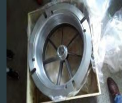
Permanent Mold A356-T6 Aluminum 20" and 24" Diameter housing
