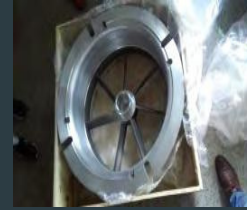
Permanent Mold A356-T6 Aluminum 20" and 24" Diameter housing
